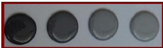
Fig. 6. Examples of prepared black glazes (5, 3, 2.5 and 1% of black pigment).
